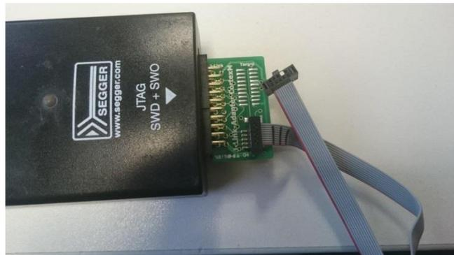
Figure 2 - J-Link Debugger and its SWD Connector
